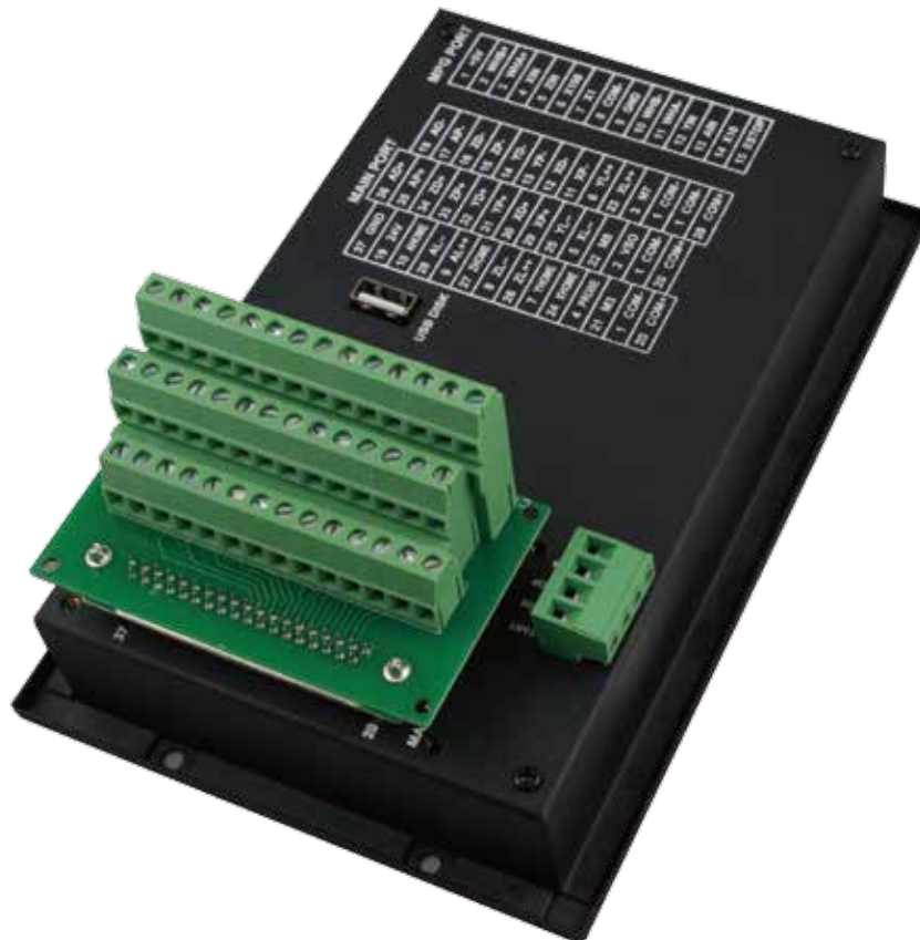
Picture 2-8 Main Port with wiring terminal
