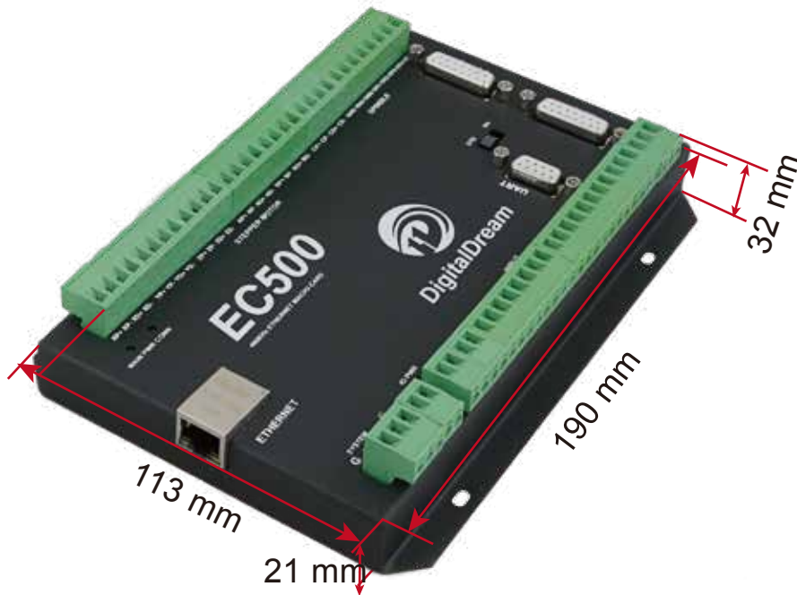
Picture 3-1 EC500 Front Appearance and size
